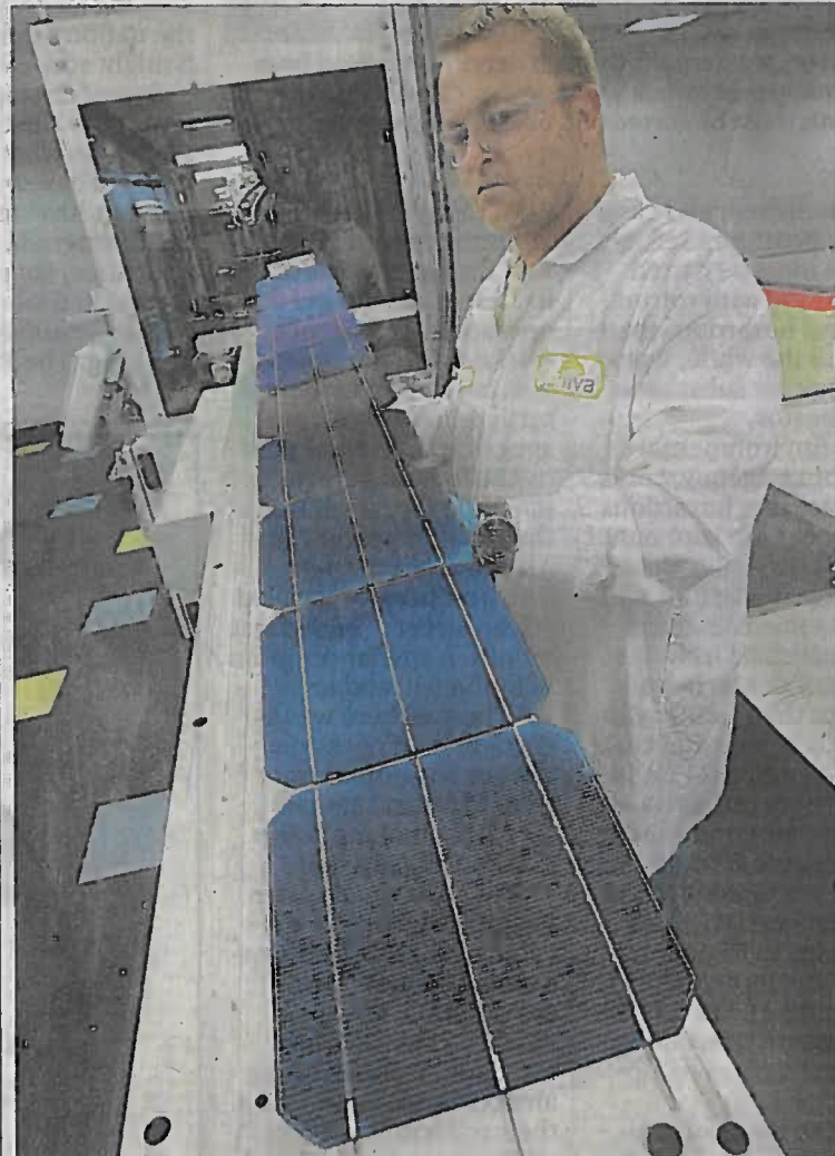
Module lab tech James O'Bryant strings finished solar cells together at Suniva. With the help of metro-based businesses, Atlanta's economic future could be tied to globalization, high-tech innovation and green biosciences. Track a solar panel from Atlanta to China, A12 Curtis Compton ccompton@ajc.com
